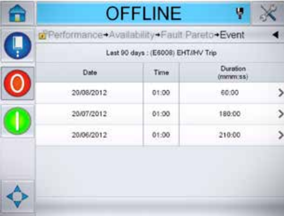
Drilling down to reveal the date, time and duration of each fault.
