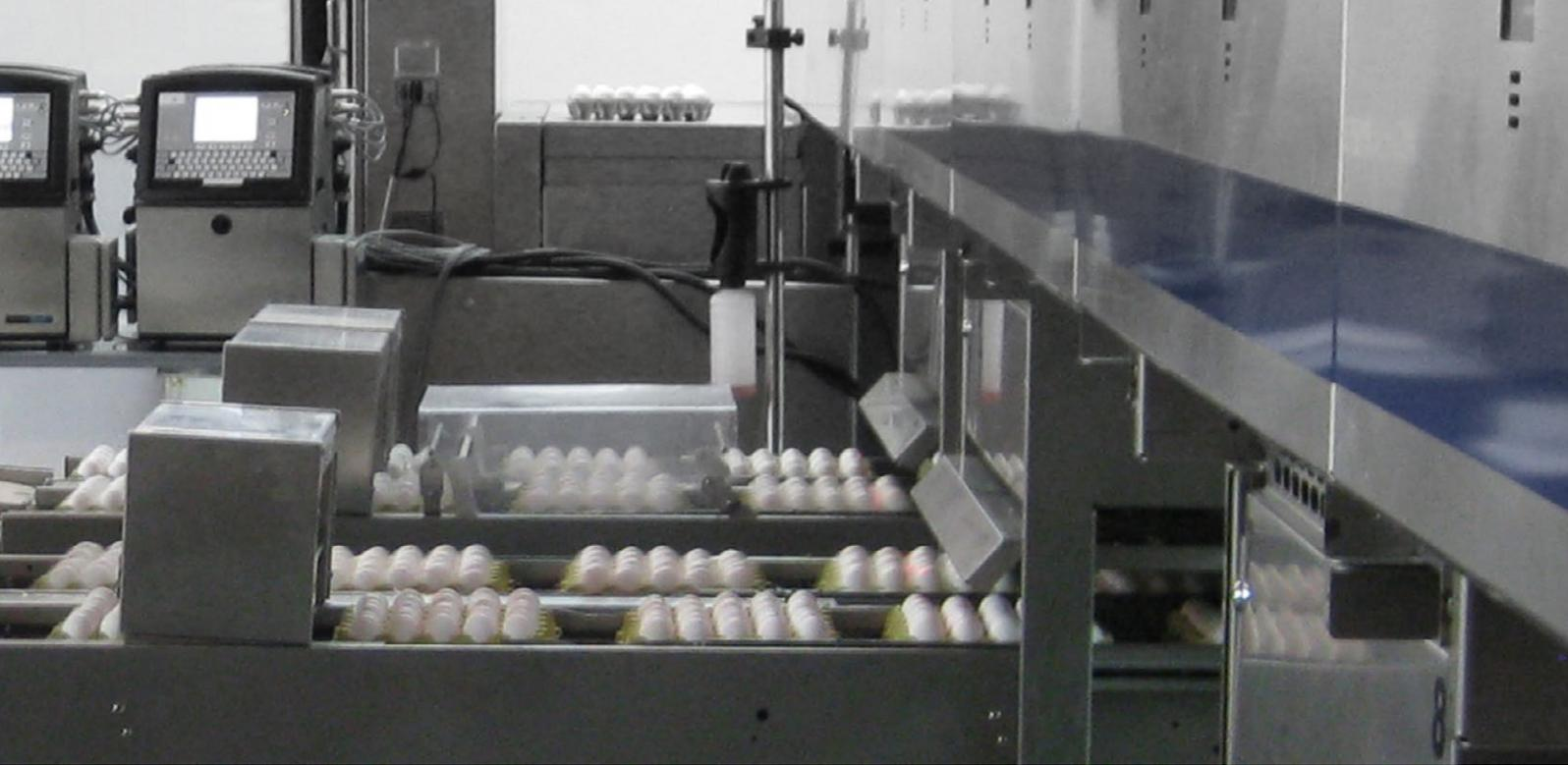
In most cases, printing equipment that is integrated directly with the grading equipment will maximize the results of your significant grader investment. For older existing grading equipment, understand that there may be additional grader investments required. Work closely with the grader manufacturer to understand the integration options. Tight grader integration is beneficial, because the grader will control the printing equipment directly and will ensure the right code is on the right egg.
