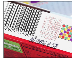
Illegible and misplaced code
