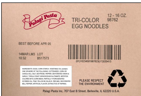
Pre-printed logos and company data. Label with ingredient listing. Product information printed in-line with ink jet printer.
